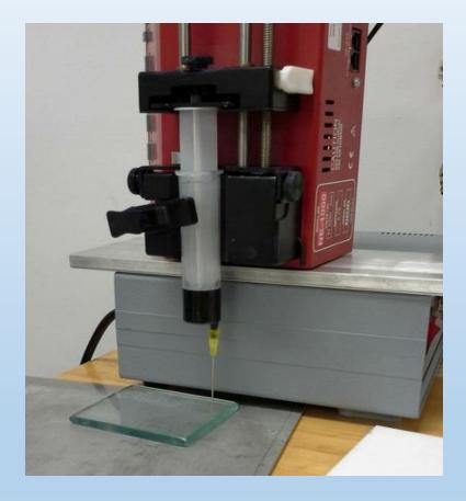
Sam Yang CNT Reinforced Ceramics 3D Printer
