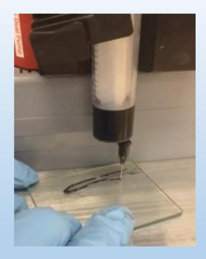
Sam Yang CNT Reinforced Ceramics 3D Printer
